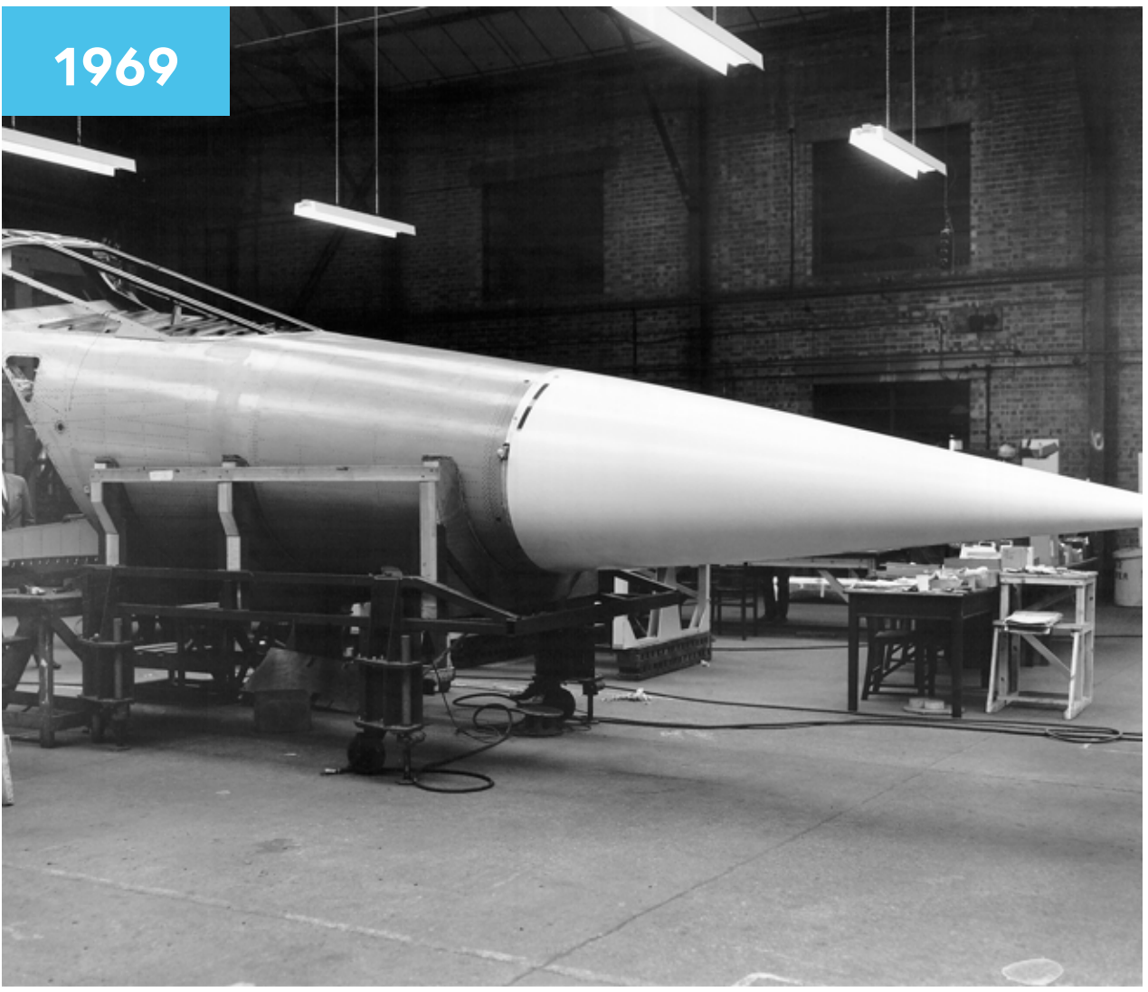
Marshall was asked by the British Aircraft Corporation to design and manufacture the Concorde droop nose.
